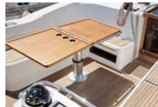
The cockpit table can be folded out and the height can be adjusted electrically (optional) or manually (standard)
