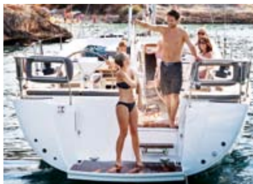
The bathing platform can be lowered manually and features a shower and stainless-steel ladder on the side, which leaves the front of the platform freely accessible
