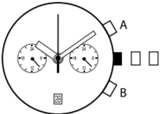
3. Press button A or B to reset the dual time of 24 hour hand to "0" position.
