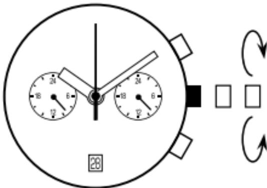
1. Pull out the crown when the second hand is at the 12 o'clock position.
