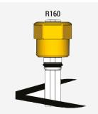
Before screwing the R160 valve, verify that the plastic paddle does not interfere with the parts inside the seat, it is necessary to have a free space of at least 35 mm. If any interference is present, cut the exceeding part of the paddle with a shear.
