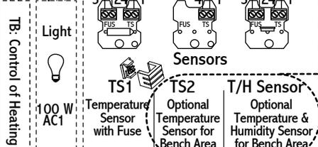
**Note:** Do not connect both Optional Sensors same time. Only one of the optional sensors at a time is allowed.
