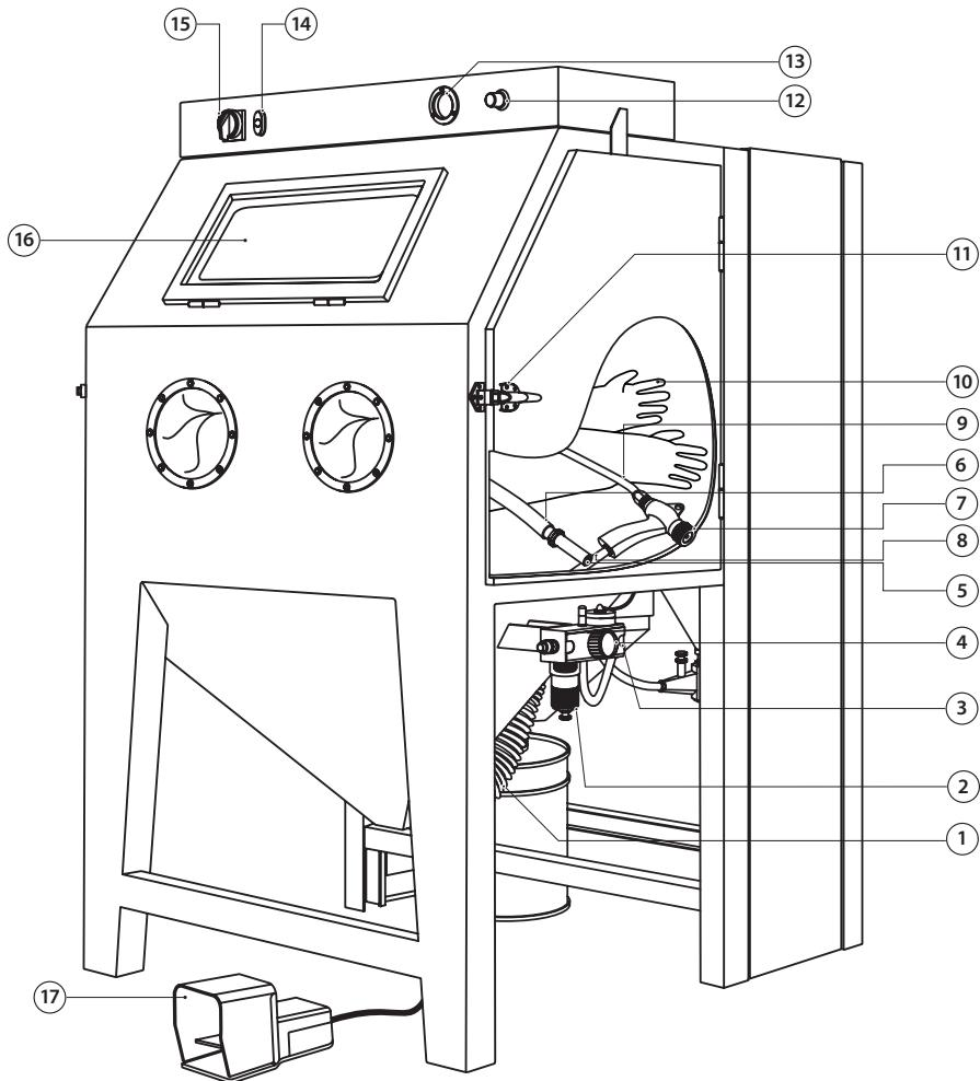
**Picture 2.0.1.** Cabinet components overview CAB-110S/135S (Front view)
