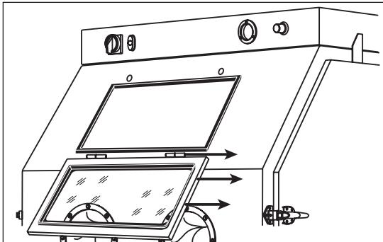
Remove the old window by pulling the window molding. Install the window molding in the window opening by fitting the narrow slit of the molding over the metal edge of the opening.
