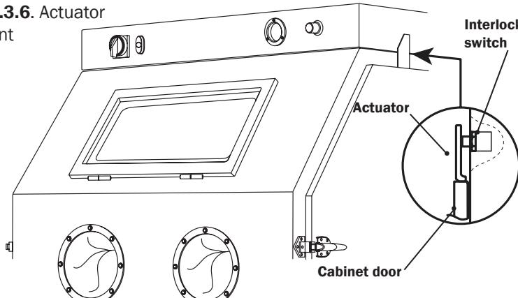
Test the operation with the doors both open and closed. Point the nozzle away from the door when it is tested, and only open the door enough to disengage the interlock switch.
