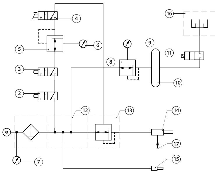
**Picture 7.4.** Pneumatic circuit diagram CAB-110S/ 135S
