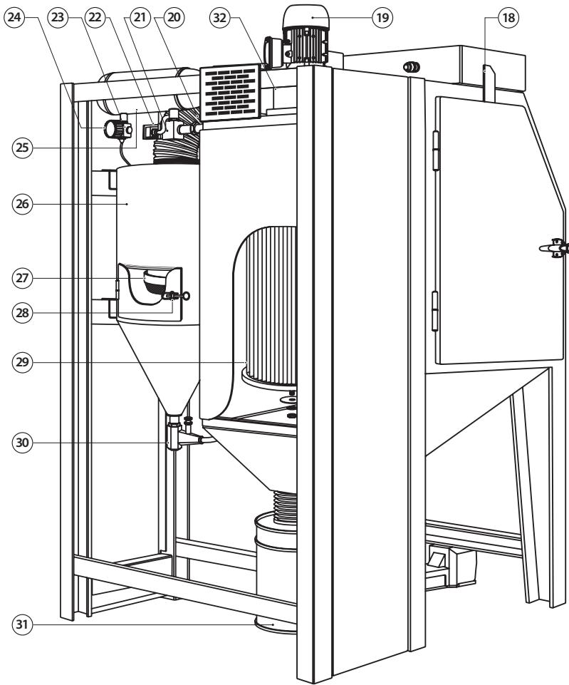
**Picture 2.0.2.** Cabinet components overview CAB-110S/135S (Back view)
