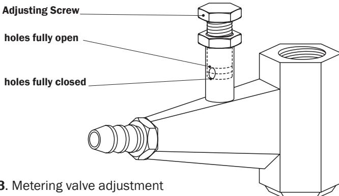
**Picture 4.3.3.** Metering valve adjustment
