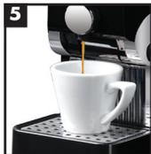
Place a second time the large cup under the coffee nozzle, push again the coffee button to re-fill the cup.
