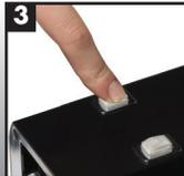
3 Press the ON/OFF button (B) for one second. The red light will switch on.
