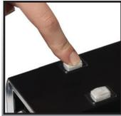
If you wish to turn off the machine manually, without using the Shut-Off Device, press and hold pressed the ON/OFF botton for **5 SECONDS** (B).
