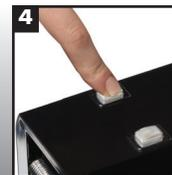
**4** Press the ON/OFF button (B) Wait until the green lamp The red lamp light up. light up (A)
