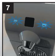
Touch one of two coffee buttons: both lights start blinking. When machine is ready to brew coffee, buttons stop blinking and become steady.
