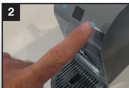
Touch and hold long coffee button (G), for 3 seconds, when you remove the finger, button (G) blink fast and pump start working. At this time machine is programming mode (machine is brewing coffee).
