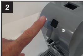
Touch and hold espresso coffee button (F) for 3 seconds when you remove the finger, button (F) blink fast and pump start working. At this time machine is programming mode (machine is brewing coffee).
