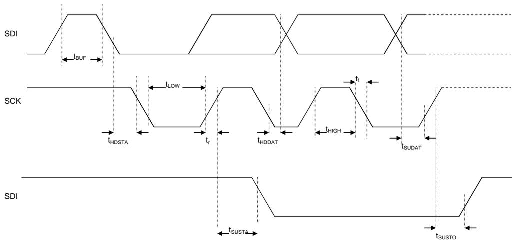
Figure 14: I<sup>2</sup>C timing diagram
