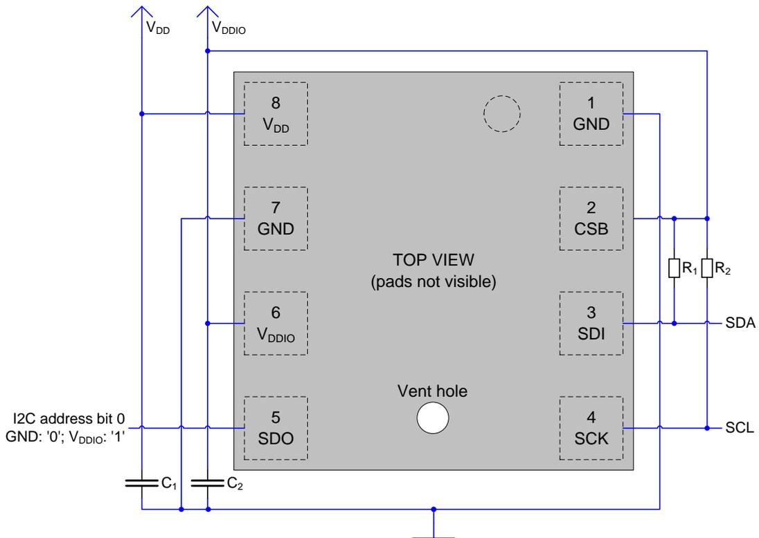
Figure 17: I<sup>2</sup>C connection diagram
