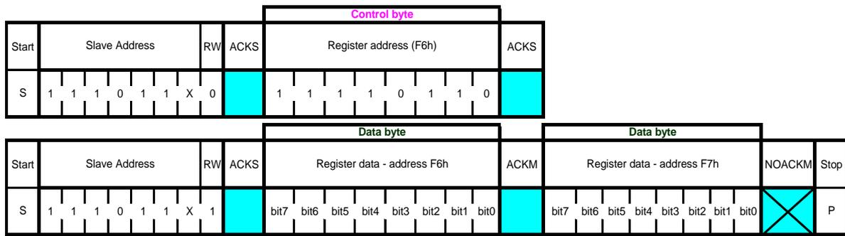
Figure 10: I<sup>2</sup>C multiple byte read
