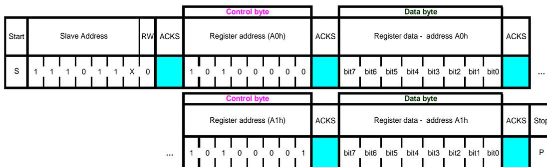
Figure 9: I<sup>2</sup>C multiple byte write (not auto-incremented)
