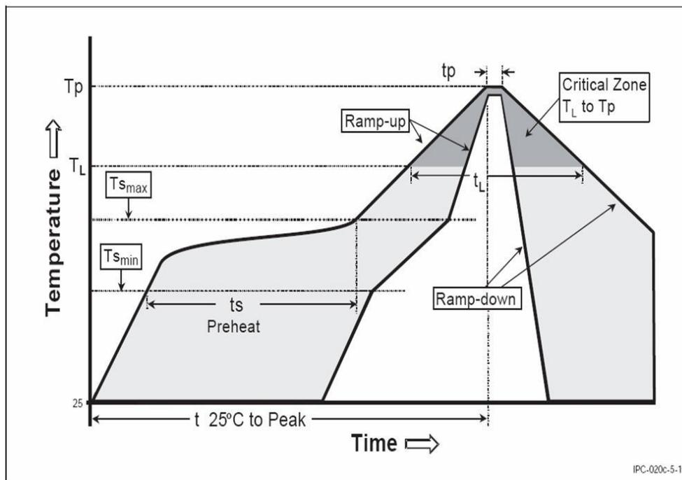
Figure 22: Soldering profile
