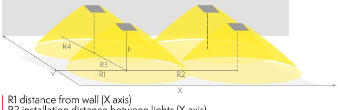
R1 distance from wall (X axis) R2 installation distance between lights (X axis) R3 installation distance between lights (Y axis) R4 distance from wall (Y axis) TWT8651WK
