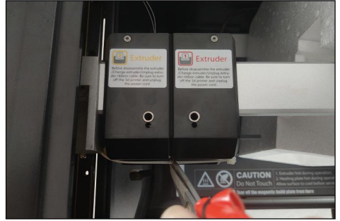
8. Cut the extruder fixing tie.
