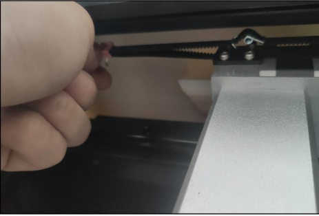
7. Remove the clamp on the right Y-axis belt.
