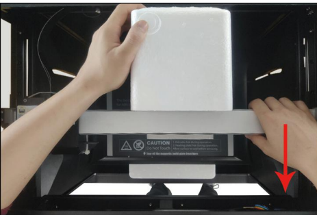
11. Move extruder to the front side and take out the foam.
