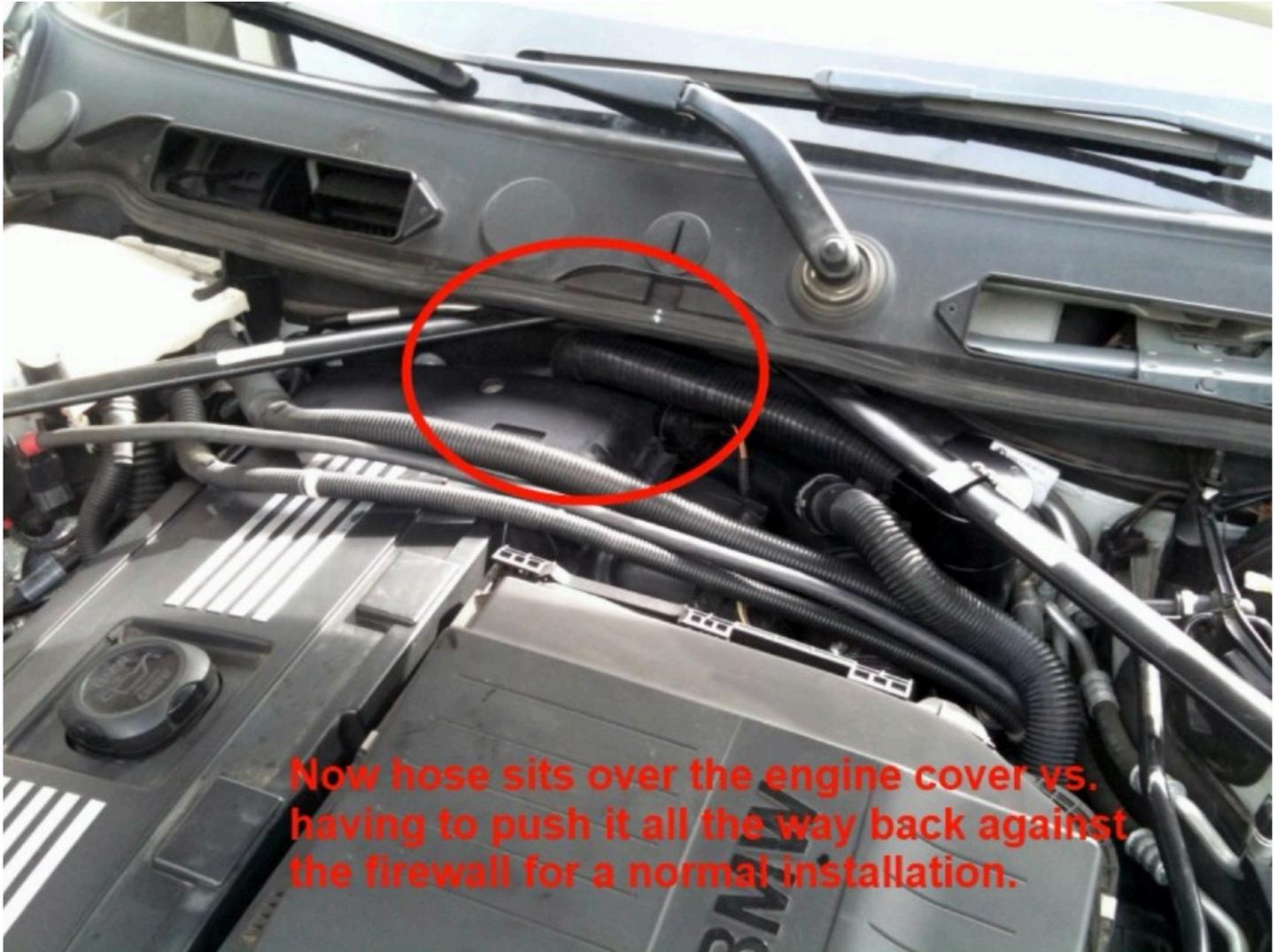
Once the engine cover is installed you can reinstall the cowl and cabin filter. Installation is complete!
