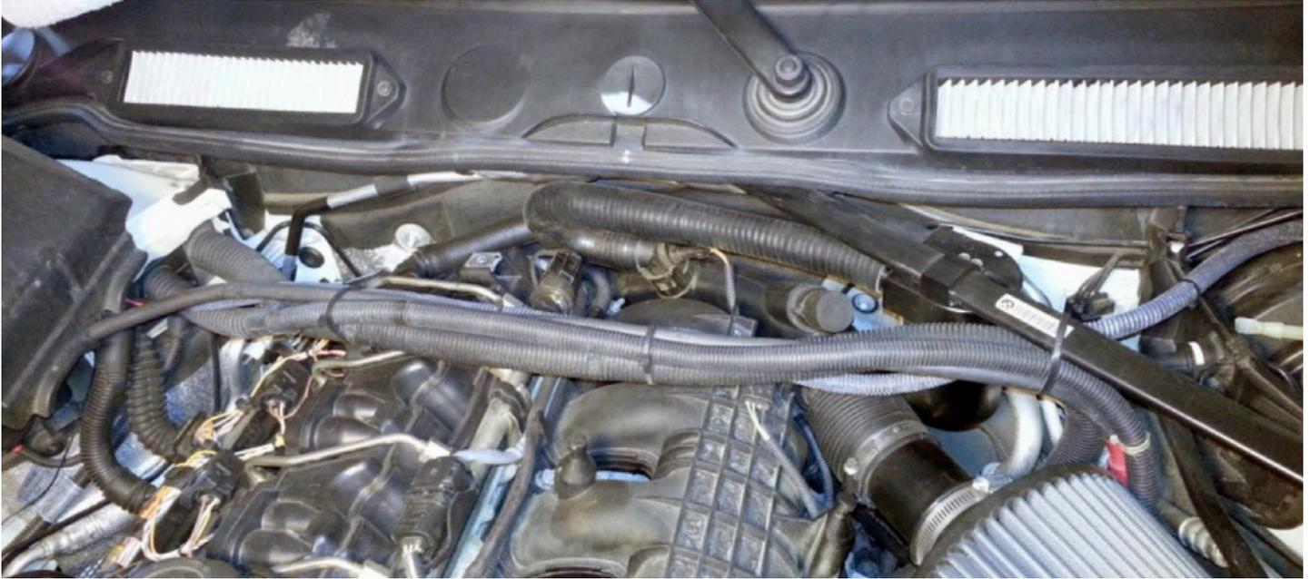
Holding the DV line out of the way swing the OCC under the strut brace and attach using the included allen screws and bracket. Only one screw is required to hold the OCC up but both can be installed.
