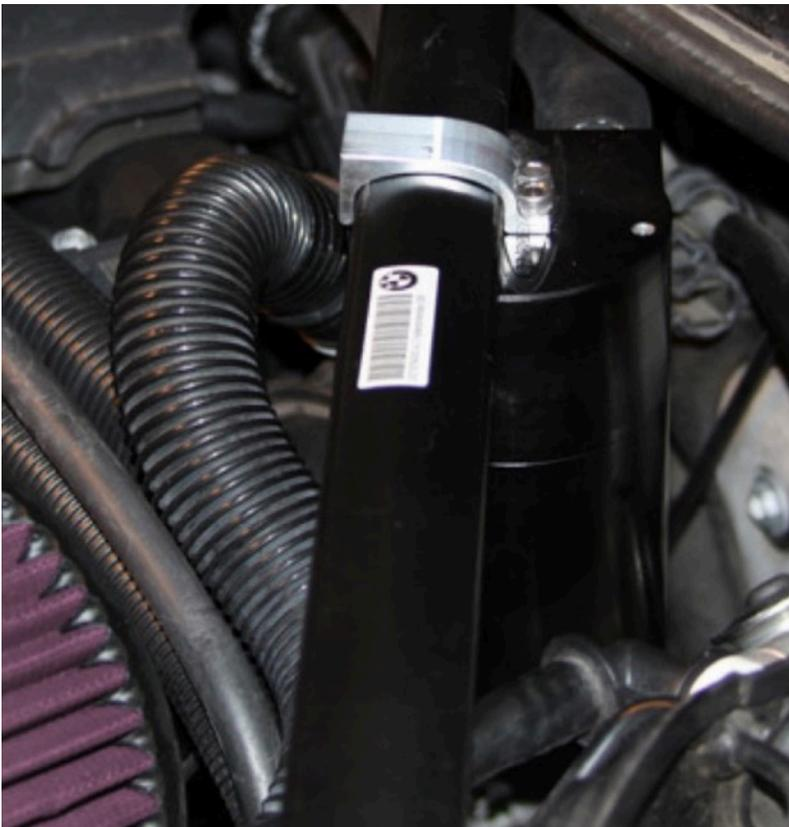
We suggest trimming the plastic engine cover slightly as shown to allow a little extra room for the OCC hose. Use a hacksaw, cutoff wheel, or similar.
