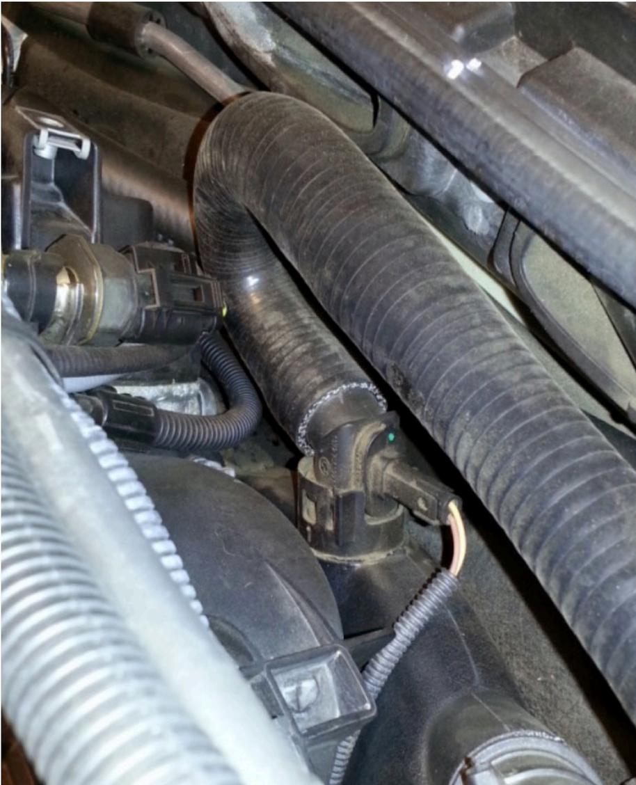
Push the UBEND over the OEM nipple as shown. The fit will be snug but ensure it's fully seated. No clamp is required. If you are unable to get the hose over the nipple use a heat gun or hair drier to heat the hose end up a bit making it more pliable. This hose will go to the "OUT" fitting on the catch can. (the side with the baffles)
