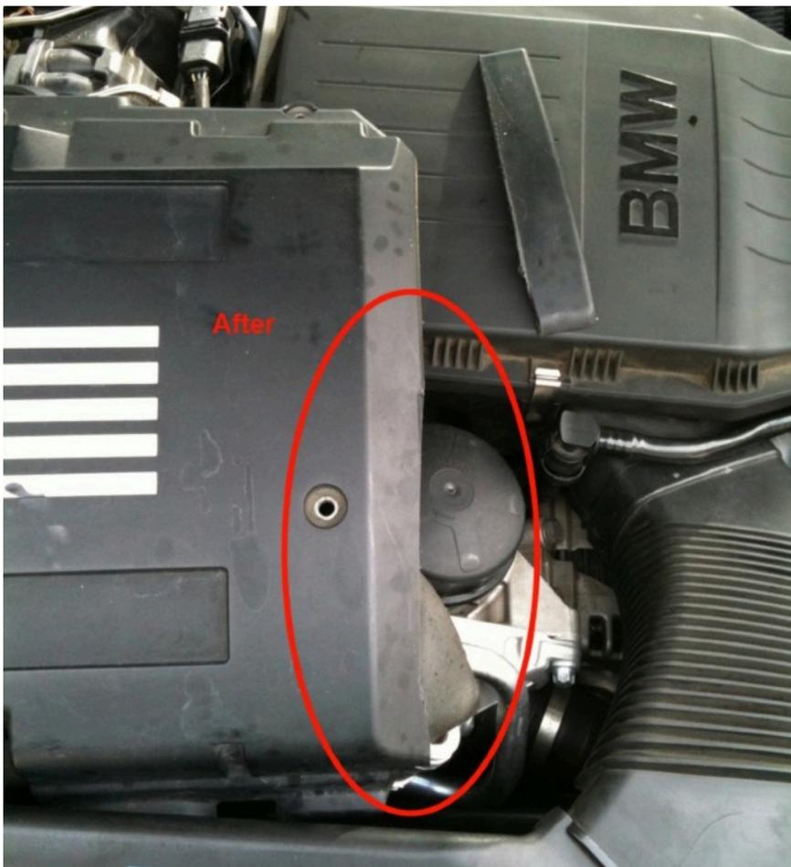
Reinstall the engine cover. It will slightly touch the rear UBEND hose and may require a bit of force to push it back in to place and align the four 5mm allen bolts. If you find it difficult to reinstall one or both of the rear allen bolts they can be left out. Spend a little extra time here to ensure you do not "fold over" the UBEND blocking flow when reinstalling the engine cover.
