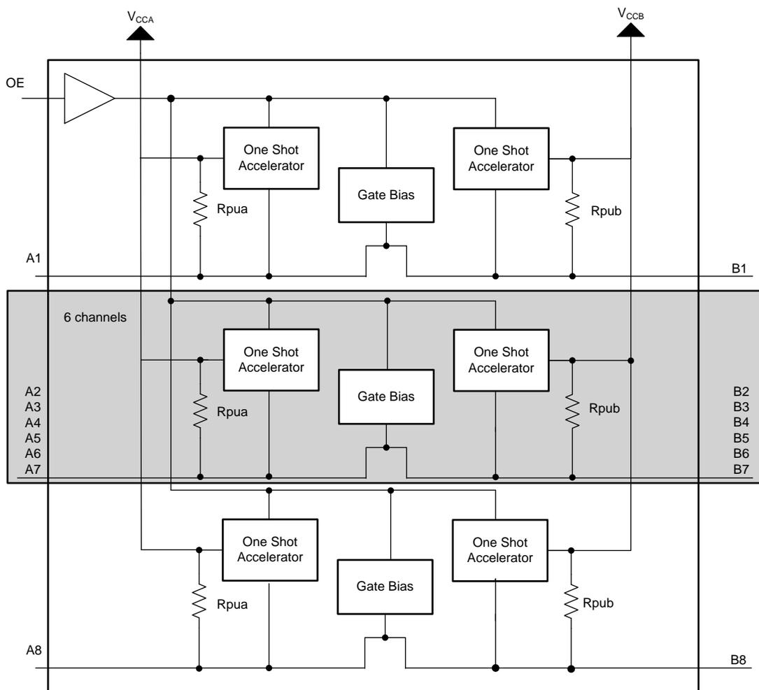
Each A-port I/O has a pull-up resistor ( $R_{PUA}$ ) to  $V_{CCA}$  and each B-port I/O has a pull-up resistor ( $R_{PUB}$ ) to  $V_{CCB}$ .  $R_{PUA}$  and  $R_{PUB}$  have a value of 40 k $\Omega$  when the output is driving low.  $R_{PUA}$  and  $R_{PUB}$  have a value of 4 k $\Omega$  when the output is driving high.  $R_{PUA}$  and  $R_{PUB}$  are disabled when OE = Low.
