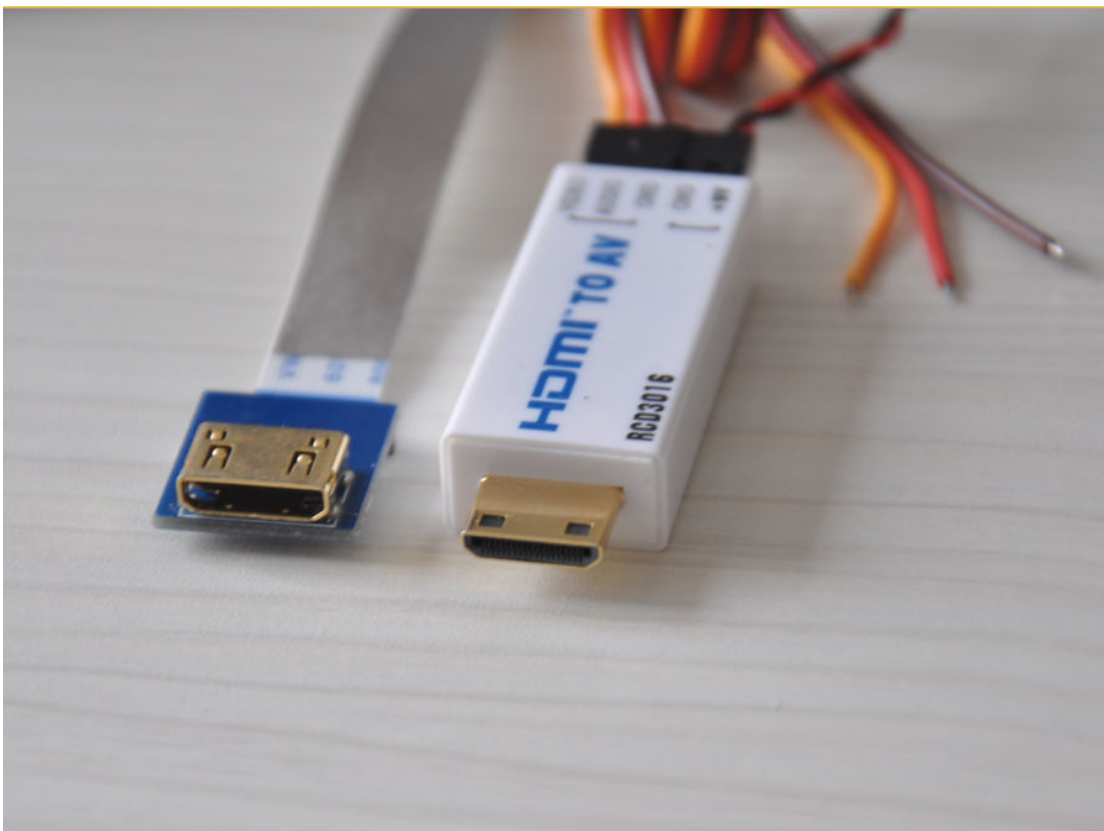
Applied HDMI mini male output (HDMI type C), it comes with a HDMI standard soft flat cable, one end of the cable is HDMI mini female connector (HDMI Type C female), the other end can be MINI or MICRO HDMI male connector, it depends on the requirement of the customer.
