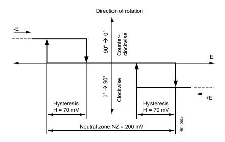
The diagram shows the relationship between the differential voltage E = Y - U (difference between setpoint Y and actual value U) and the direction rotation, including hysteresis and neutral zone.
