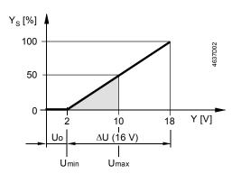
Max. positioning range Ysmax =  $100 \% (95^\circ)$  Span Ys =  $50 \% (47.5^\circ)$  Offset Uo = 2 V Span  $\Delta \text{U}$  = 16 V
