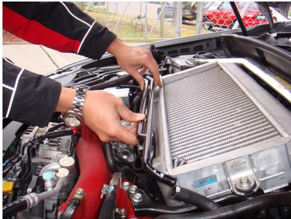
5. Using the provided 1/2" tee piece, connect the standard oil breather lines on the left hand side of the intercooler in the orientation shown in the picture below and run the provided 1/2" hose under the intercooler to the oil breather line on the other side of the intercooler, using the provided 1/2" straight joiner to join the rubber hose to the existing breather line on the right hand side.
