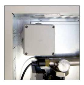
The wiring case has all the connections required for the regulation unit: boiler enable signal (NO), room thermostat (TA), safety thermostat (TS) and pump power (POMPA). It has to be powered at 230V.
